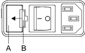
The fuse holder (A) with the mains input fuses is located next to the mains switch.
