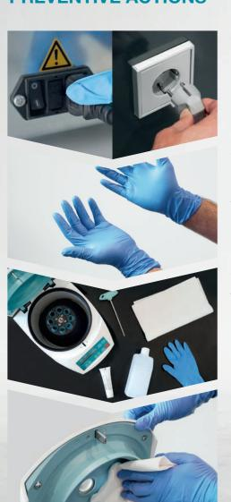
Switch off the device and disconnect the centrifuge from the power supply.
