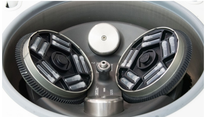
ZentriMix-Rotor carrying vial adapters for 2 ml Screw Cap Micro Tube. Each rotation unit carries two adapters which lie on each other. Only the adapters on top are visible.
