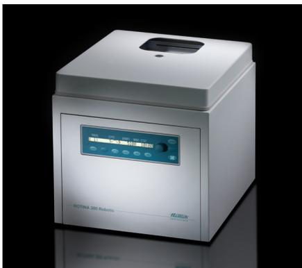
**Flexible and Versatile:** The **ROTINA 380** automated centrifuge is available with or without temperature control in a benchtop or under-bench version capable of centrifuging microtiter plates and blood collection tubes. The ROTINA 380 RC is ideal for an automated workstation in routine clinical diagnostics. The intended use is for standard clinical samples, as well as the preparation of cellular and bacteria samples.
