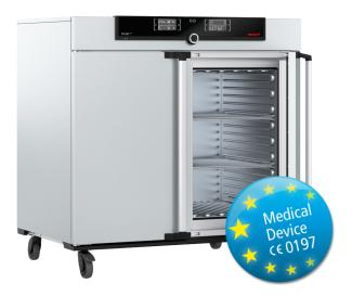
The indispensable safety feature for this hot air steriliser: Setpoint Wait. This means that the programme for sterilisation only starts when the set temperature has been reached. This feature can also be used with freely positionable Pt100 temperature sensors. Here the sterilisation time only begins when the set temperature has been reached at all measurement points, and reliable sterilisation is guaranteed at all times.
