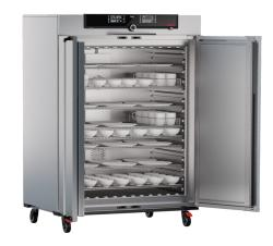
The Memmert heating oven dishwasher UF750DW is specially adapted to the EN50242 standard and complies with the standard's specifications.
