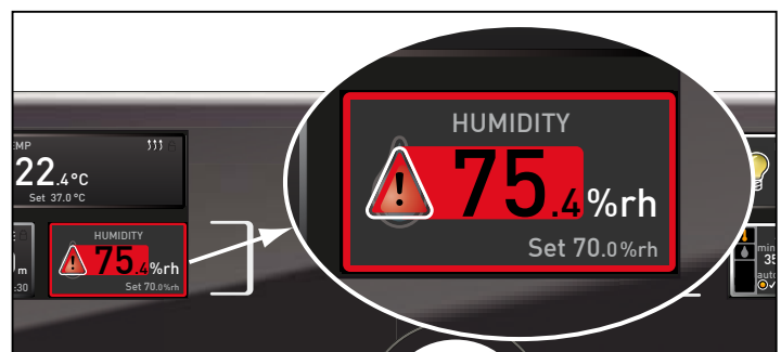
Fig. 22 Humidity monitoring triggered
