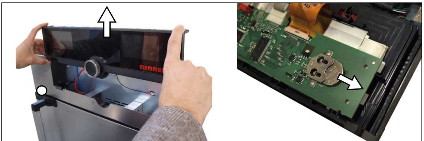
Fig. 32 Removing the lithium battery
